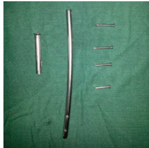
Fig. 2: The broken device, an 11 mm diameter Simplified Universal Nail, with a transverse break at the proximal static interlocking screw hole, while all 4 screws were intact.
