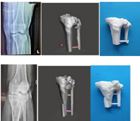
Figure 1: Left: Plain radiograph. Center: Digital modelling. Right: 3D printed model
