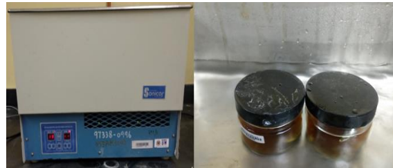
Figure 2: Image of sonicator and the air-tight container in ultrasound bath.
